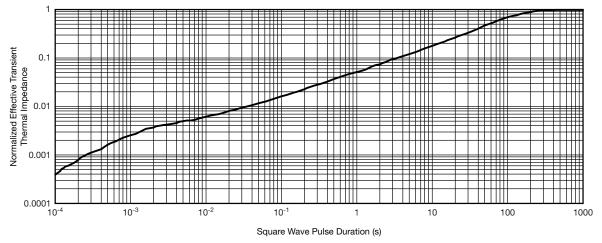
Normalized Thermal Transient Impedance, Junction-to-Ambient
