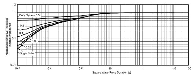
Normalized Thermal Transient Impedance, Junction-to-Case
