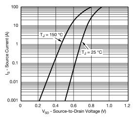
Source Drain Diode Forward Voltage
