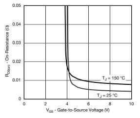
On-Resistance vs. Gate-to-Source Voltage
