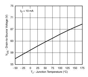
Drain Source Breakdown vs. Junction Temperature
